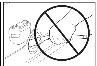
Figure 28 Incorrect Removal of Charger DC Plug
