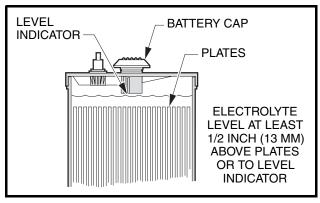
Figure 26 Battery Electrolyte Level
