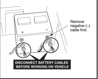
Figure 1 Battery Cable Removal - Electric
