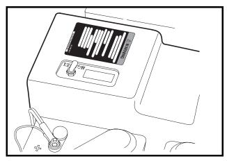
Figure 10 Tow/Run Switch
