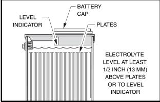
Figure 29 Gasoline Vehicle Battery
