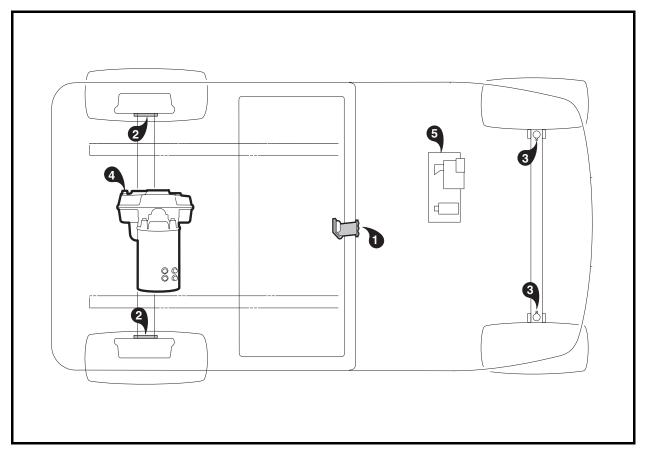
Figure 24 Lubrication Points – Electric Vehicles
