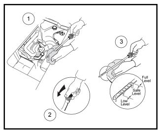
Figure 31 Engine Oil Level Check
