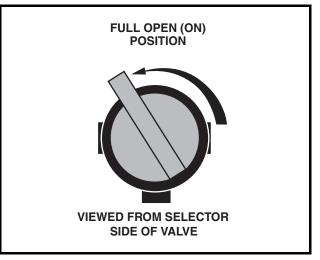
Figure 21 Fuel Shut-off Valve - Open Position
