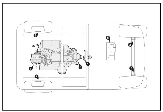
Figure 25 Lubrication Points - Gasoline Vehicles
