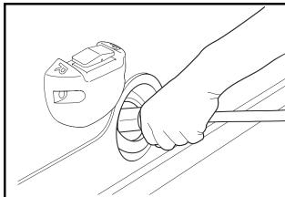
Figure 27 Correct Insertion of Charger DC Plug
