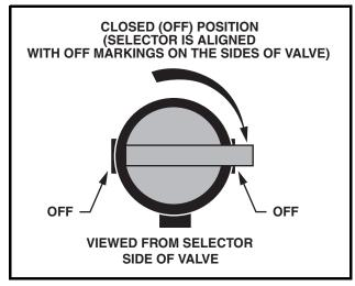
Figure 20 Fuel Shut-off Valve - Closed Position
